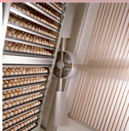
Separate heating, cooling and ventilation controls per incubator section of 19,200 hen eggs.
