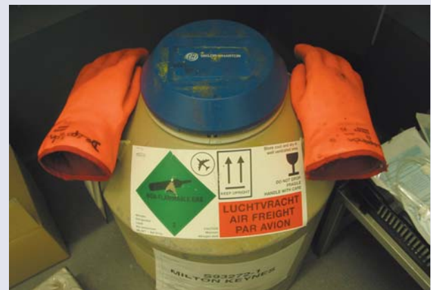
Figure 1: Correct storage of the cell associated MD vaccine in liquid nitrogen is essential to the viability of the vaccine.
